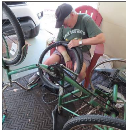
Replacing Old Tube
